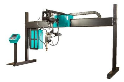
The machine is designed to rebuild track shoes of all models. It is of very robust and rigid construction and is designed to weld the lug/bar on to the grouser, without removing it from the track chain.
