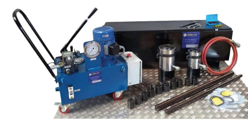
Single acting return hydraulic jacks are available in both alloy steel and aluminium and have 50 and 100mm stroke which pin, and bush can be replaced in one or multiple strokes. Jacks are centre hole type and are places on C-sleeves (one over the other) through which centre rod passes and nuts are tightened at the ends. Tie rods and nuts are machined from an alloy steel material, hardened, and tempered to increase strength and toughness.
