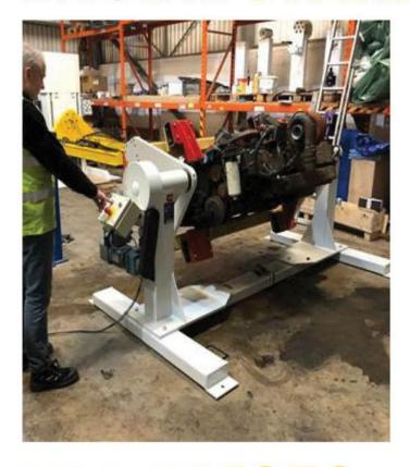
HEMS supply specialised engine rotating stand packages including all necessary adaptor plates, for all engine and transmission makes and models that are currently available on the market.
