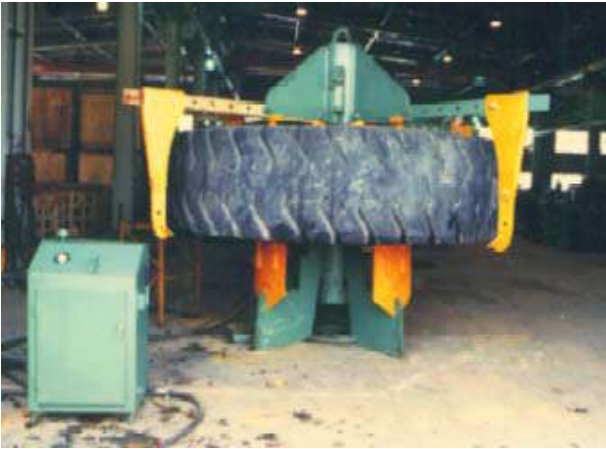
Fig. 2 The grapple head lifts the tire and rim assembly by means of an overhead crane and is placed onto the ram of the stand. The 4 lower demounting shoes are positioned to hold the lower side ring.
